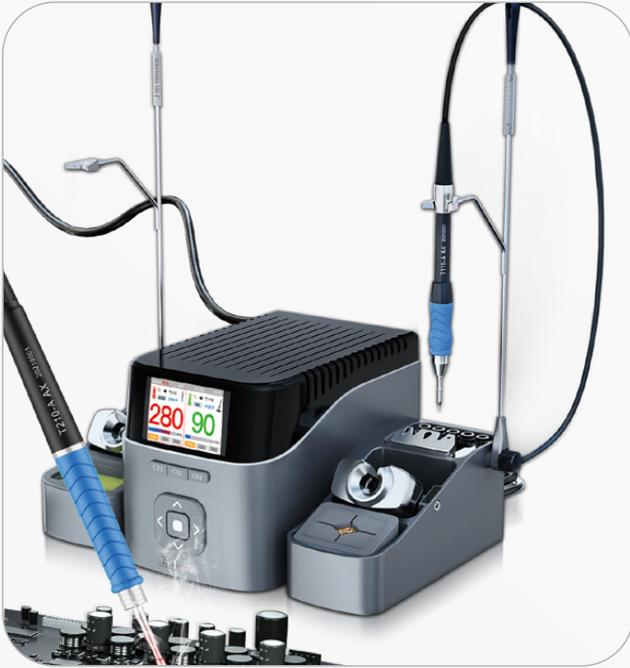
The dual channels of the soldering station can work separately or simultaneously. When the soldering pen is picked up from the holder, the iron tip will automatically heat to the selected temperature. You can start the job
