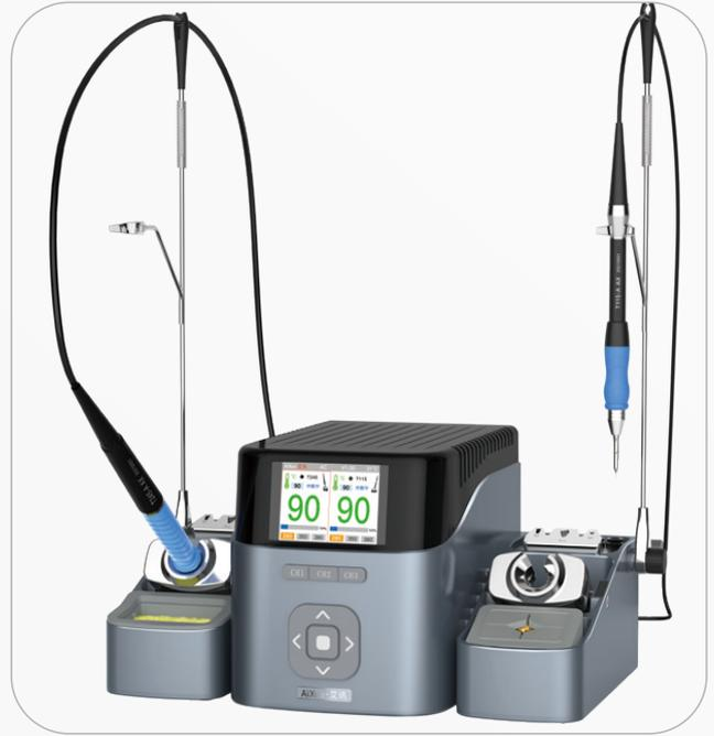
When the soldering pen is placed in the Standby seat or suspended on the Standby rack, the host will automatically enter the Standby mode and the temperature will automatically drop to the preset Standby temperature.
